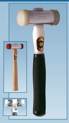
With chrome plated zinc heads (except 720N) Thorex Hammers are fitted with two durable white nylon faces or with two medium red plastic faces. Nylon hammers have the option of either wood or plastic handles. All hammers can be fitted with fibreglass handles to special order.
