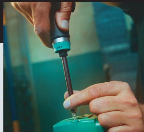
The TiN Bit is based on a titanium nitride coating, which produces a high surface hardness up to 2500HV. It is produced by utilizing the CVD method. The precise fit and micro-rough surface ensure a secure fit in the screw. The minimized ejection forces and high surface hardness makes the TiN Bit optimally suited for long-term industrial use. The perfect bond between steel and coating ensures a long service life
