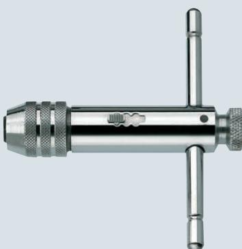
The tap wrench with ratchet is very versatile. The chromed all-steel design withstands even the highest loads. The precise and smoothly running T-handle ensures the optimal balance between pressure and lateral guidance. The clamping jaws are carefully hardened and the right-left rotation and lock gears with steel slider ensure smooth functioning in each area of application.
