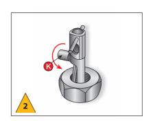
Turn knurled knob (**K**) to extend blade (**B**) into a thread groove on an undamaged section and tighten by hand only.
