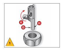
Turn knurled knob (**K**) to fully retract the blade (**B**) into housing (**H**). Insert **Nes Internal** tool into the threaded hole or bore to be repaired.
