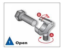
Turn handle (**A**) to raise floating blades (**B**). Place the **Nes External** tool over thread to be repaired.
