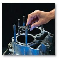
The Nes External thread restorer is available in 4 sizes and can repair threads from 4 mm (⁵/₃₂") diameter up to 152 mm (6") diameter.
