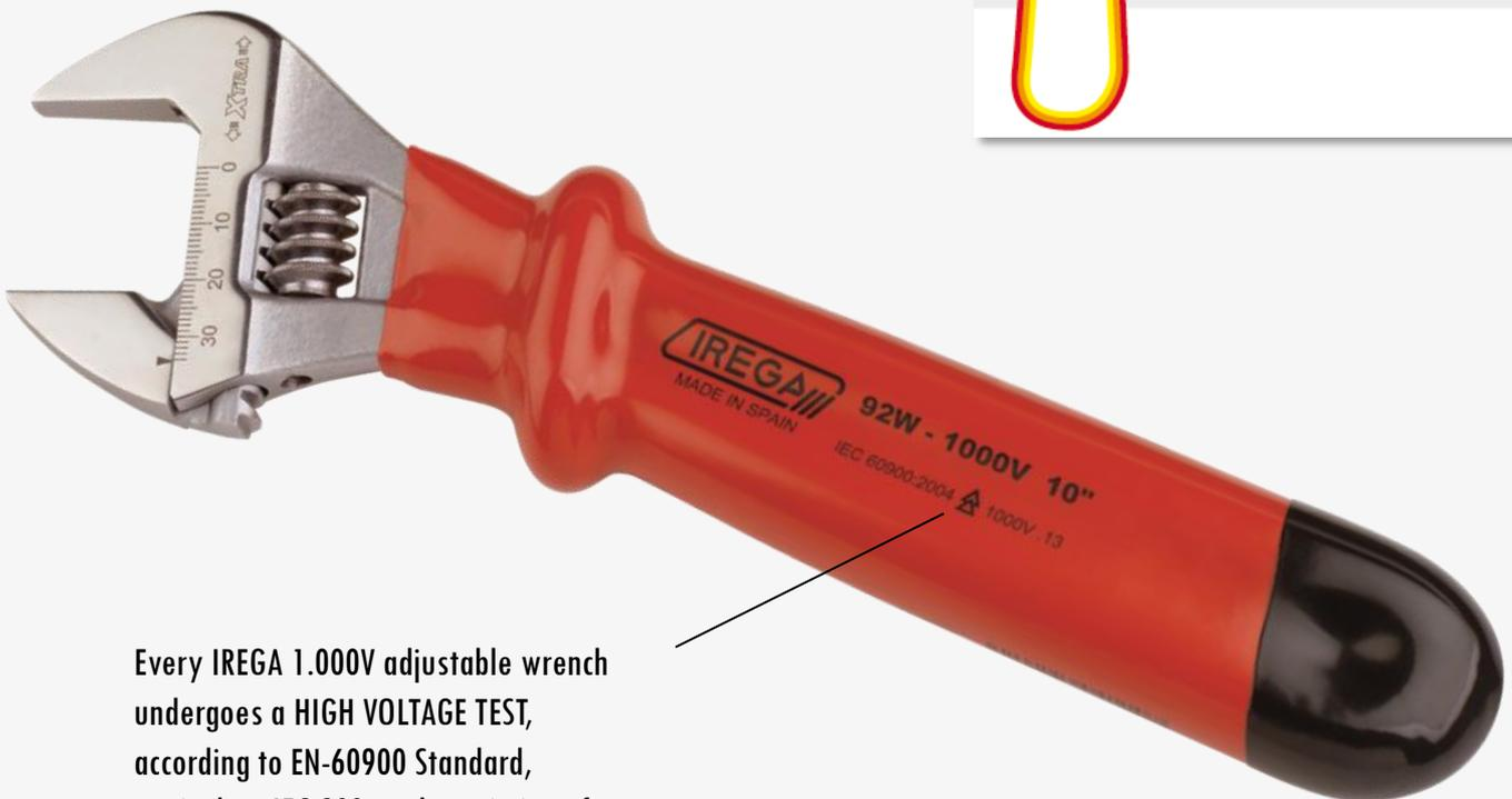
Every IREGA 1.000V adjustable wrench undergoes a HIGH VOLTAGE TEST, according to EN-60900 Standard, equivalent IEC-900, and consisting of a 10.000V charge for 10 seconds, after which there should be no damage to the handle.
